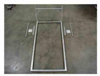
Bolt leg frame to main frame using 2-3/8"x1" carriage bolts, nuts and washers.
