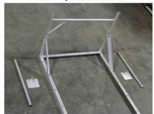
Bolt each brace on using 2 - 3/8" x 1" carriage bolts, nuts, and washers.
