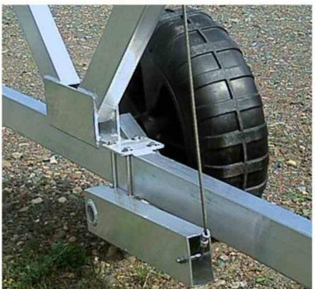
Attach the cable to the top Frame Rail and fasten using the removable link.
